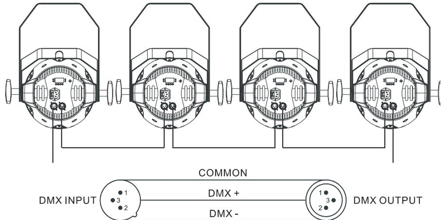
Termination reduces signal errors and avoids signal transmission problems and interference. It is always advisable to connect a DMX terminal. (Resistance 120 ohm 1/4W) between pin2(DMX-) and pin3(DMX+) of the last fixture.
