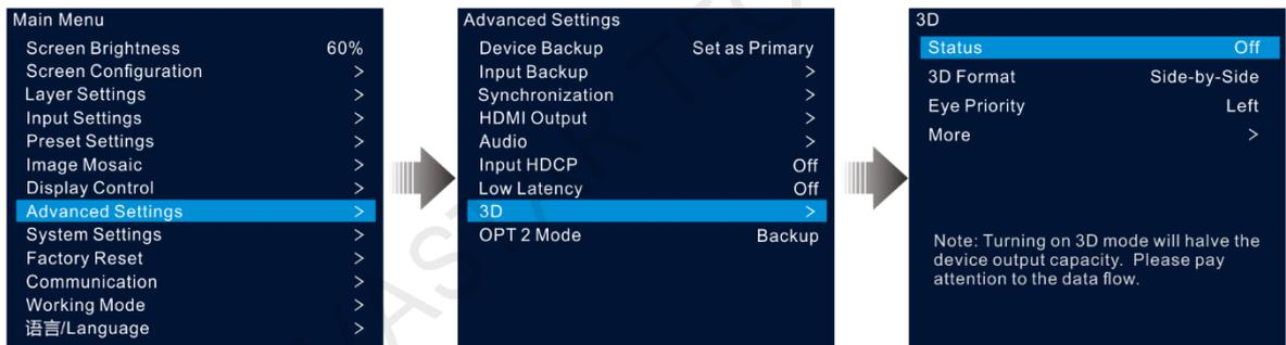
Step 2 Select the 3D format of the video source. The options include **Side-by-Side**, **Top-and-Bottom** and **Frame Sequential**.
