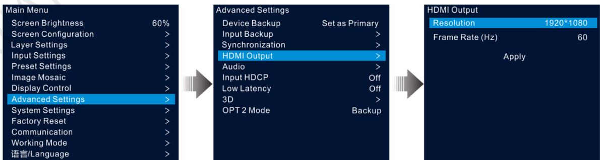
Step 2 Select **Resolution** to set the desired resolution for the connector.
