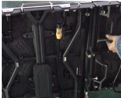
Figure 3.8 alignment hole position
