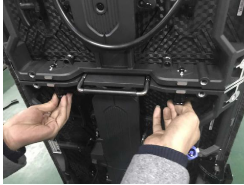
Figure 3.7 lock and tighten the Up-down fast assemble lock
