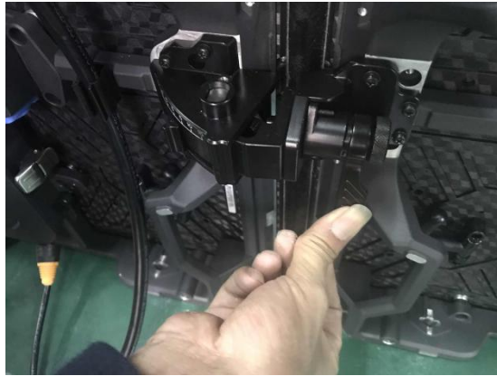
Figure 3.5 curve lock is tightened to complete radian splicing
