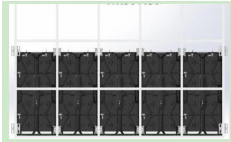
Figure .3.21 schematic diagram of the first row cabins installation
