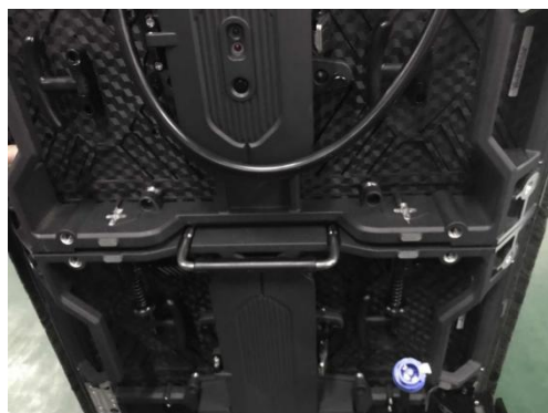
Figure 3.6 up and down Cabinet are aligned according to the positioning pin
