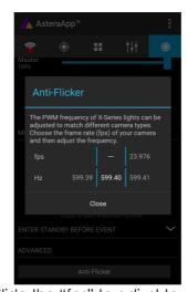
Slide the "fps" to adjust to default values for a framerate. Slide the "Hz" to fine-adjust.
