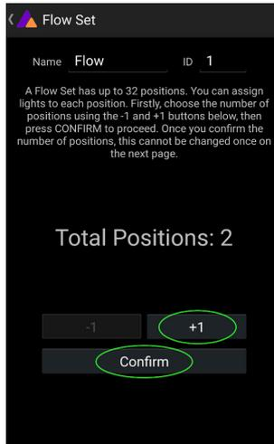
Each flow set can have up to 32 positions. Once the correct number is entered, press “Confirm”.
