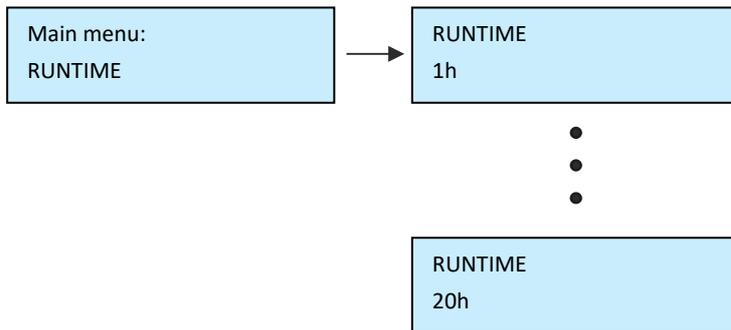
The light is able to adjust its power to meet a certain runtime on battery. The runtime is always calculated for a full battery.
