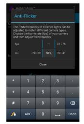
Press the highlighted frequency to enter a custom value between 200 and 1205 Hz.
