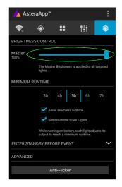
As soon as more than one Set is created Otherwise, only one slider is available. It and at least one set is currently targeted, a sub-master for each Set is shown.
