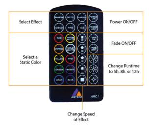
The ARC1 is very handy to switch several lights on or off at a time. The ARC1 can also accept configuration commands that are sent from the AsteraApp<sup>™</sup> to a light by pressing the POWER ON button.
