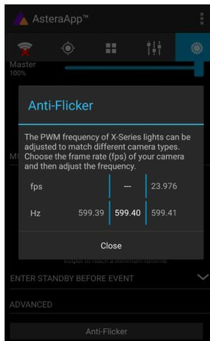
Slide the "fps" to adjust to default values for a framerate. Slide the "Hz" to fine-adjust.
